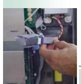
Typical skimming devices installed inside fuel dispensers (see footnote: PIN Security & AFDs)
